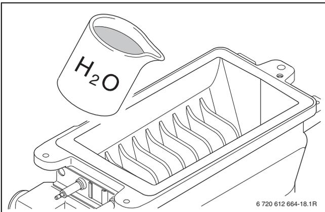
Fig. 90 Rinsing the heat exchanger
