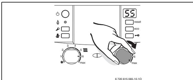
Fig. 65 Thermal disinfection
