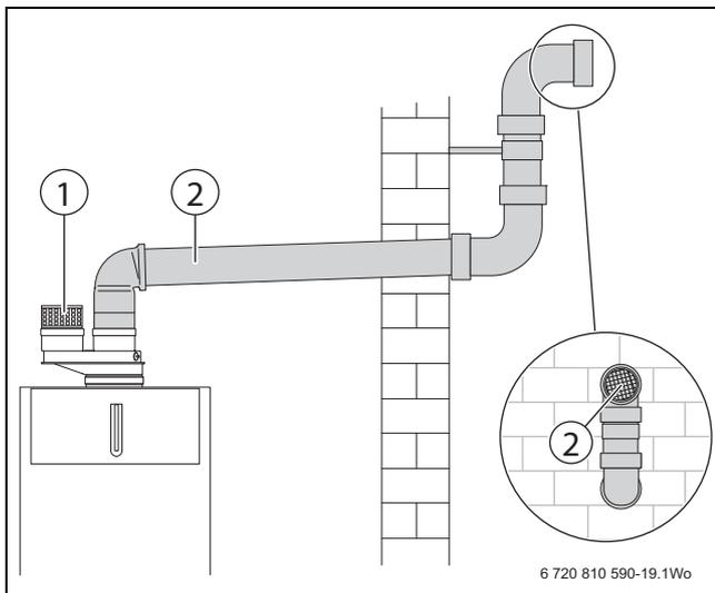
Fig. 32 Horizontal venting system (room air only)
