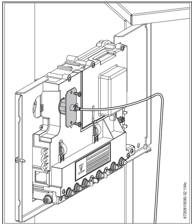
Fig. 80 Removing the boiler pressure gauge
