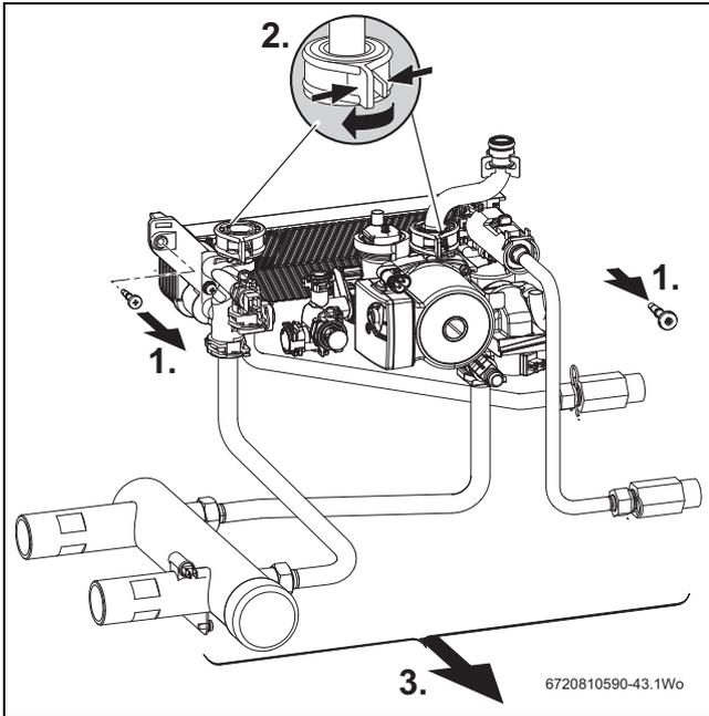
Fig. 81 Removing the hydraulic assembly
