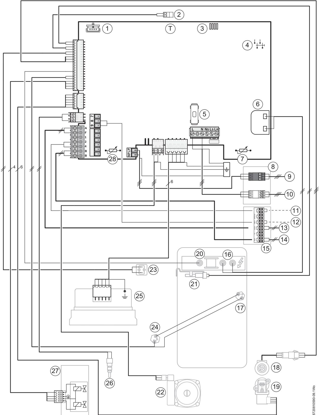
Fig. 9 Electrical wiring diagram combi boiler KWB..-3A
