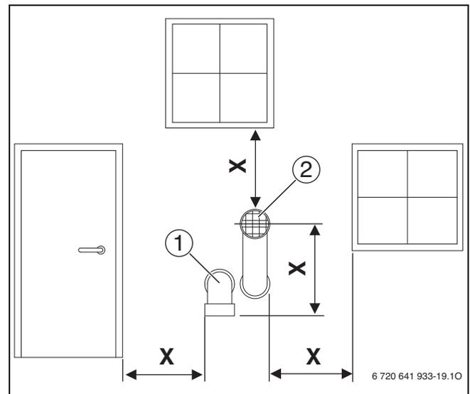
Fig. 30 Vent & combustion air pipe position of a sealed combustion system
