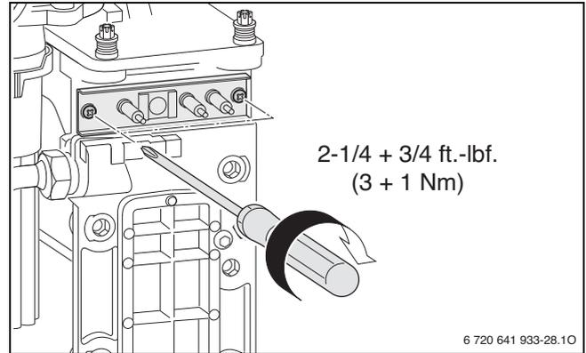
Fig. 83 Reinstalling the electrode set
