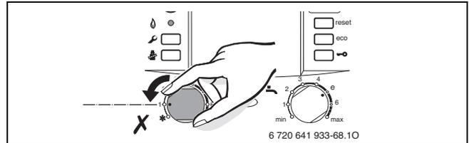
Fig. 62 Frost protection of the heating system
