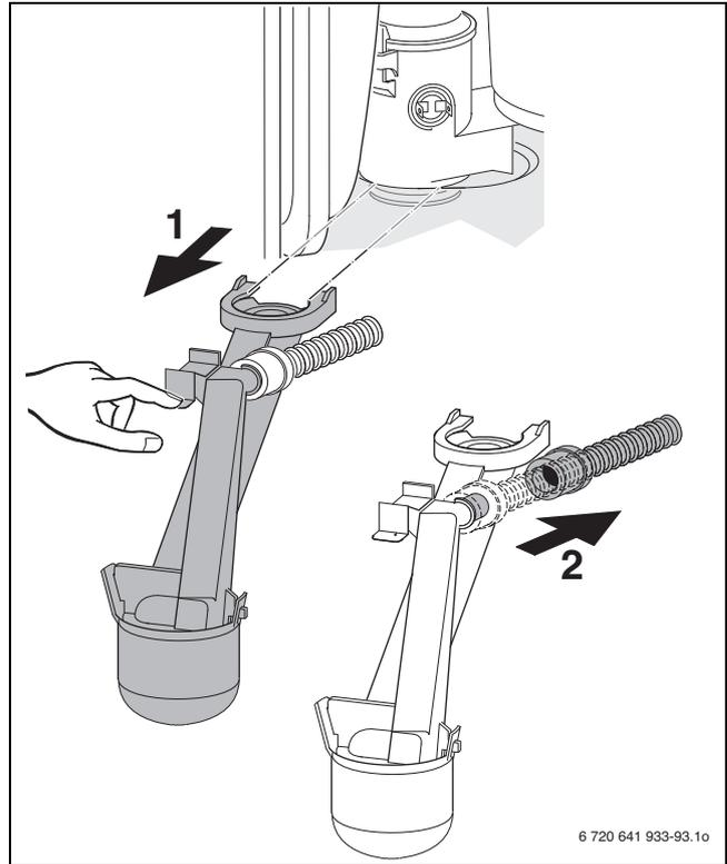
Fig. 87 Removing the condensate trap
