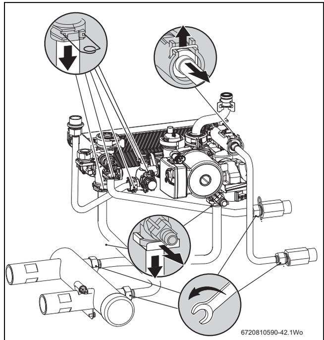
Fig. 79 Removing pipe connections
