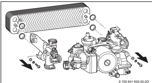
Fig. 82 Removing the plate heat exchanger
