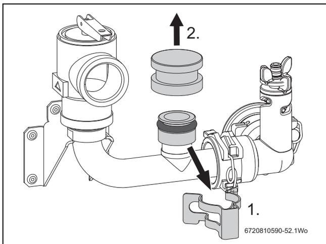
Fig. 23 Installing a LWCO device - removing dummy plug
