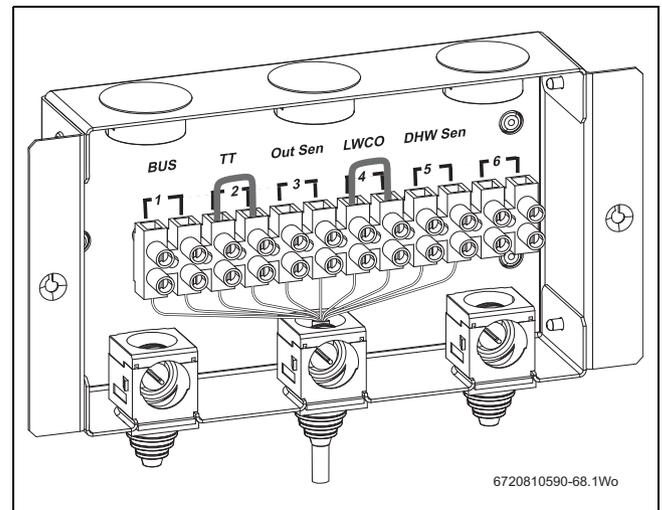
Fig. 50 Low voltage (LV) connections
