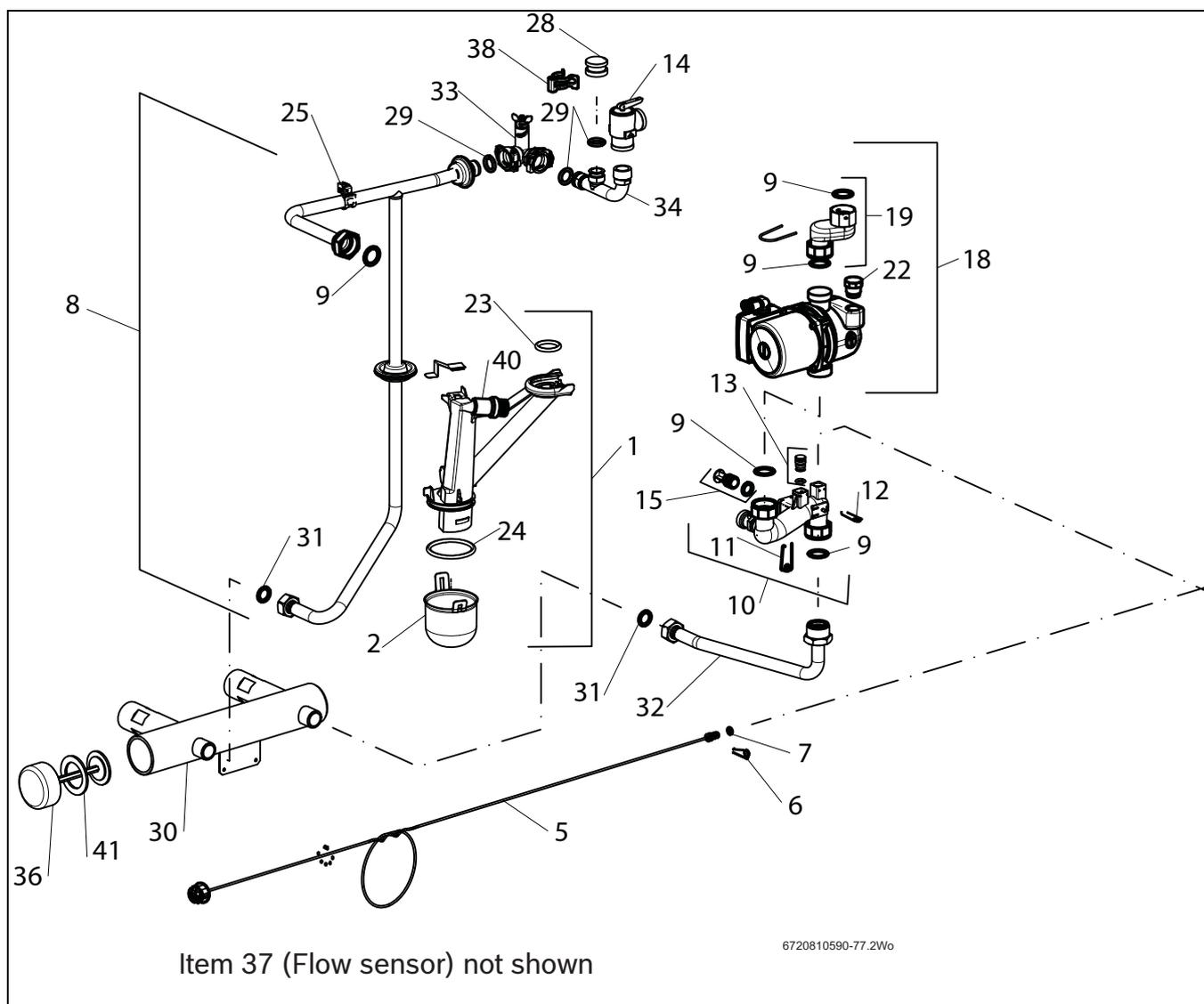
Fig. 98 Group 5 Pipes heating boiler KBR.. 3A Greenstar
