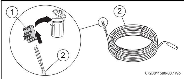
Fig. 52 DHW tank sensor connector plug removal
