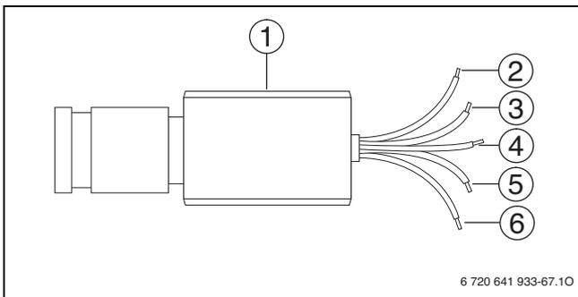
Fig. 53 Wires of a LWCO device with LWCO adapter
