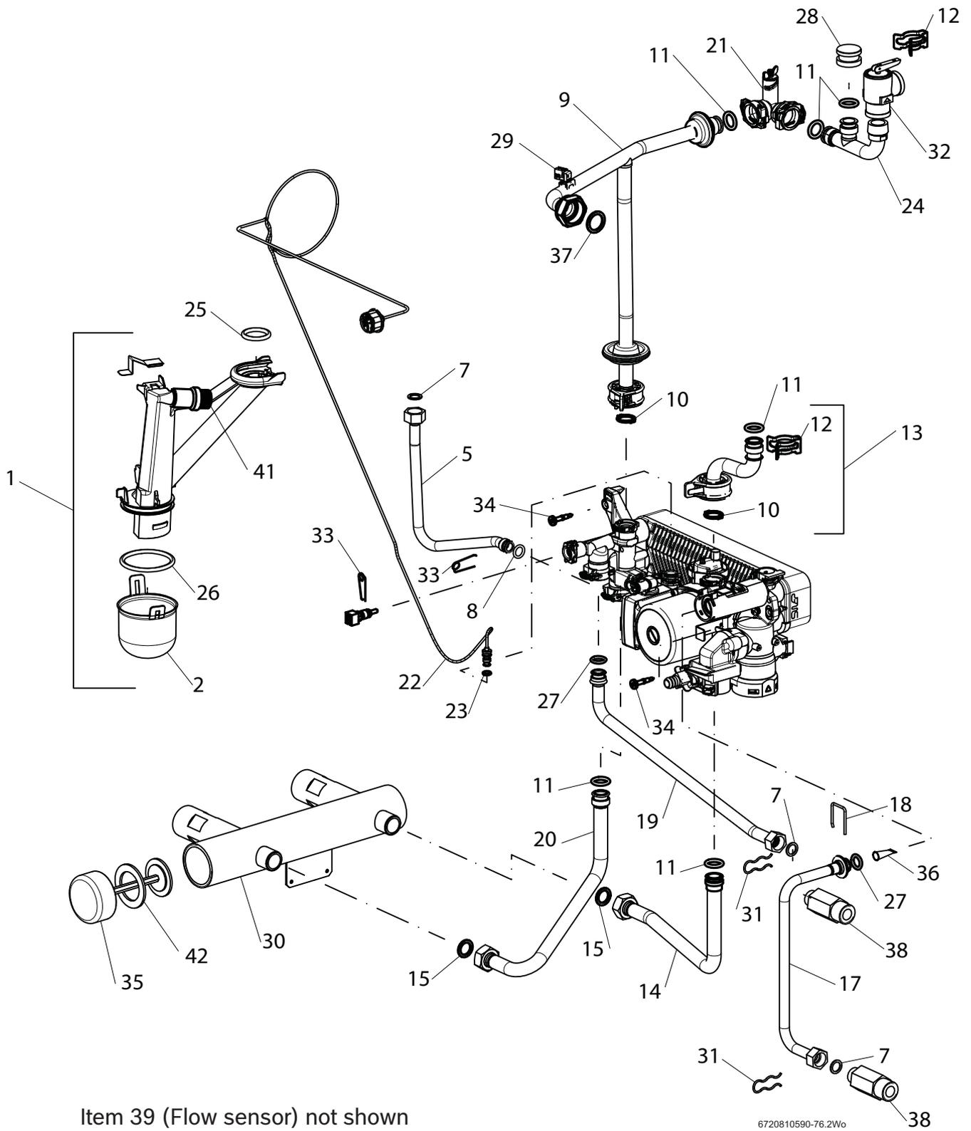
Fig. 97 Group 4 - Pipes combi boiler KWB..3A Greenstar
