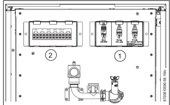
Fig. 42 Installer junction boxes with covers removed
