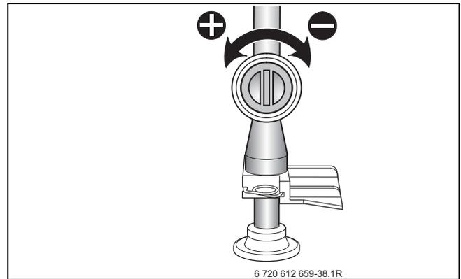
Fig. 73 Set CO<sub>2</sub> or O<sub>2</sub> level for maximum nominal output
