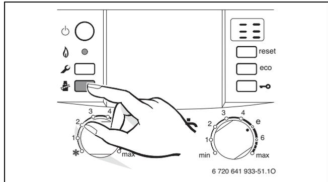
Fig. 76 Press the emissions test button
