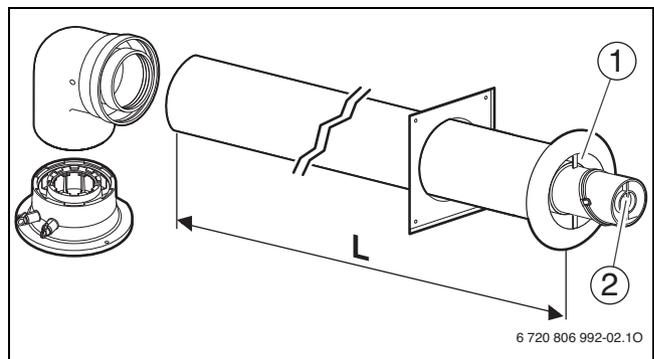
Fig. 28 Horizontal venting system (telescopic concentric vent kit)
