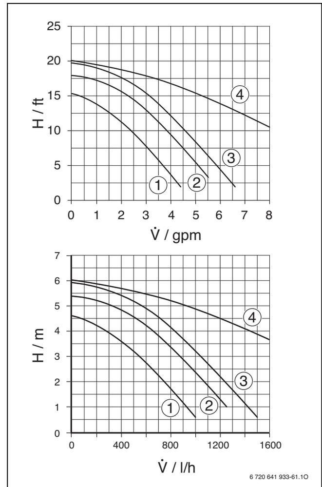
Fig. 67 Pump curve of the boiler pump combi boiler
