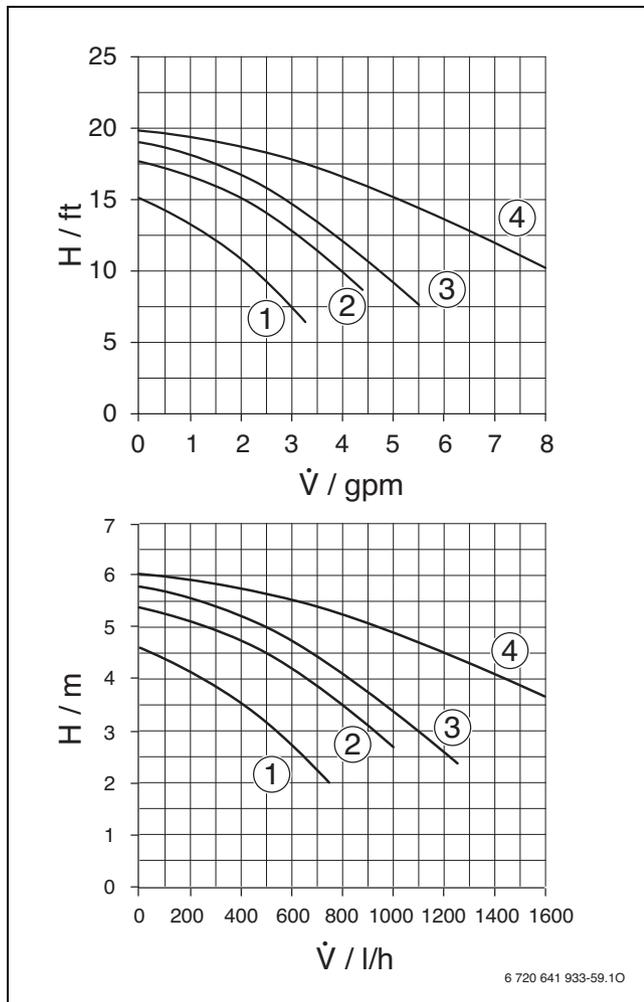
Fig. 66 Pump curve of the boiler pump heating boiler
