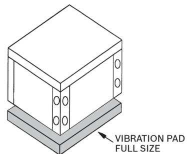
If the unit is installed on a floor over a crawl space, it should not rest on long, unsupported floor joists. Vibrations may be created in the joists with the crawl space acting as an amplifier box resulting in undesirable noise. A drain pan is recommended where water released during start-up or maintenance could cause damage below the unit.
